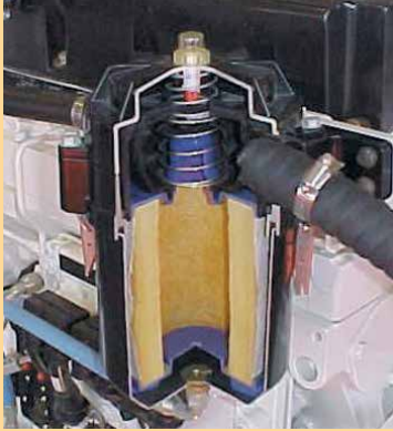
Cummins QSM11 marine engine with CCV cutaway
